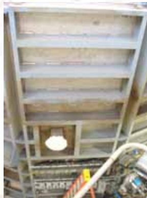
Sequoia Detector Vessel Spallation Neutron Source Project Oak Ridge National Laboratories Design analysis by Grantec Sequoia is considered to be one of the largest vacuum chambers ever built in North America
