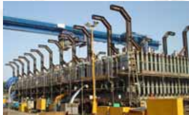
Multistage Flash (MSF) Desalination Vessel 22 tubular exchanger stages, weight 500 tons Vessel in fabrication yard in Abu Dhabi Design analysis by Grantec
