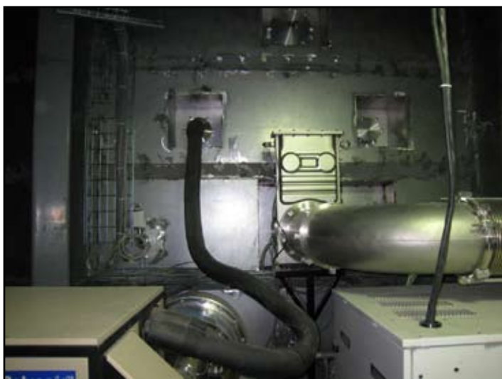
SNS Sequoia Detector Vessel wall section in way of cryogenic and vacuum pumps (pumps shown in the foreground)
